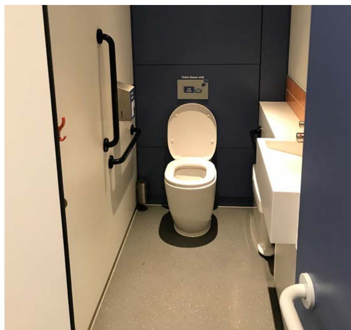
Standard cubicle with hooks, grabrails, single-sheet toilet paper dispenser and shelf; Wellcome Collection. credit: HHCD
